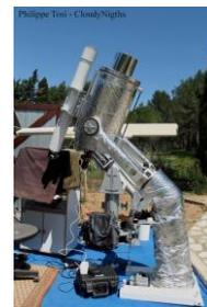
**Figure 6.** Protecting equipment from Sun with aluminum foil (credit Philippe Tosi, CN)
