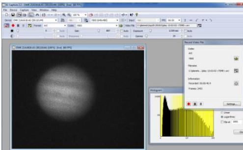
**Figure 4.** A snapshot of the PC screen during DDO of Jupiter on 2<sup>nd</sup>, Feb.2013 captured with a 0,28m/f10 telescope and a 3x Barlow.
