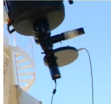
**Figure 2.** The flip-mirror helps centering the Sun (during alignment) and the planet with the eyepiece and then the observer let the light pass to the filter wheel and the camera.
